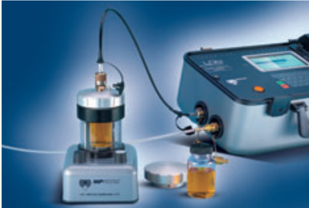
110 ml standard bottle sampler unit incorporates de-aeration facility. Suitable for mineral oil applications only.
