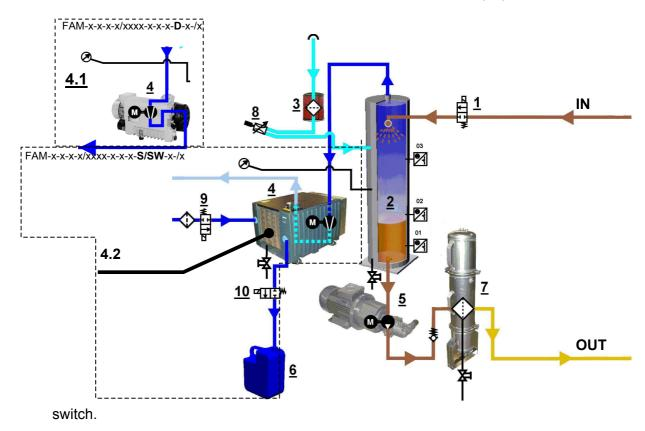
The vacuum in the reactor is regulated with the regulating valve (8).
