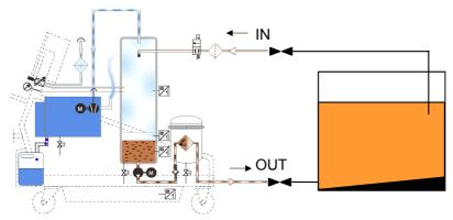
The FAM is connected with suction and pressure lines to the tank and cleans the medium to be found there in continuous operation.
