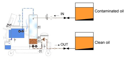
The FAM is connected to the contaminated oil tank by means of a suction line and pumps the fluid into the clean oil tank.
