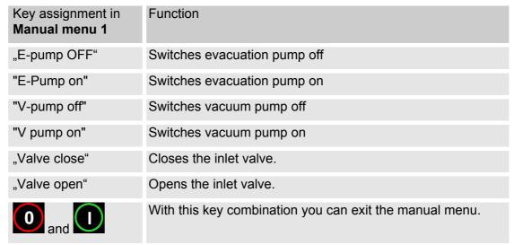
The menu for manual operation switches off automatically after 15 minutes.
